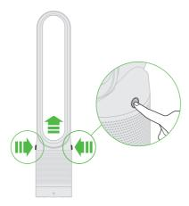
Press buttons to lift off loop amplifier and lift off filter.
